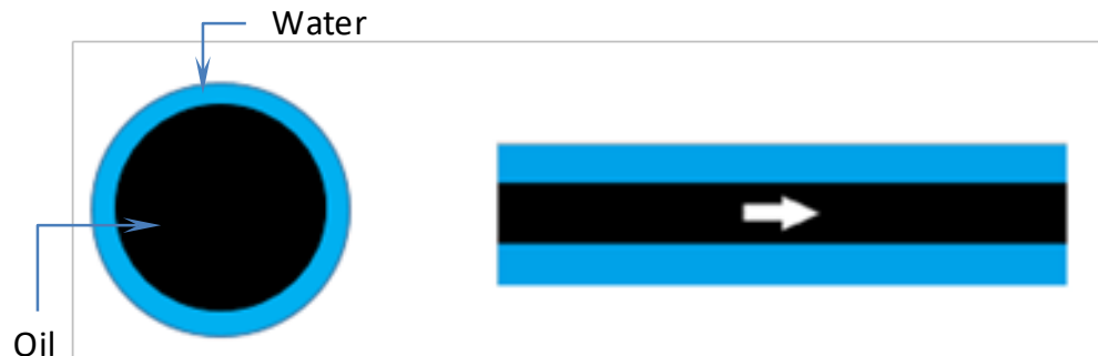
Figure 1. Schema of the two-phase (oil and water) flow via core-flow
