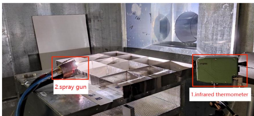
Fig. 1. Main equipment and layout of graphite purification zone
