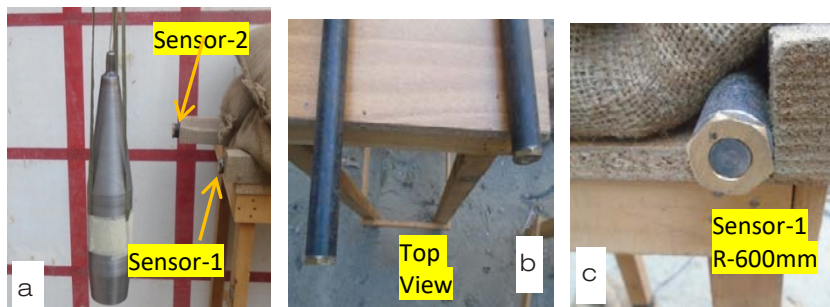
Figure 4: Setup for measuring (a) peak pressure and (b, c) close view of transducers with protection
