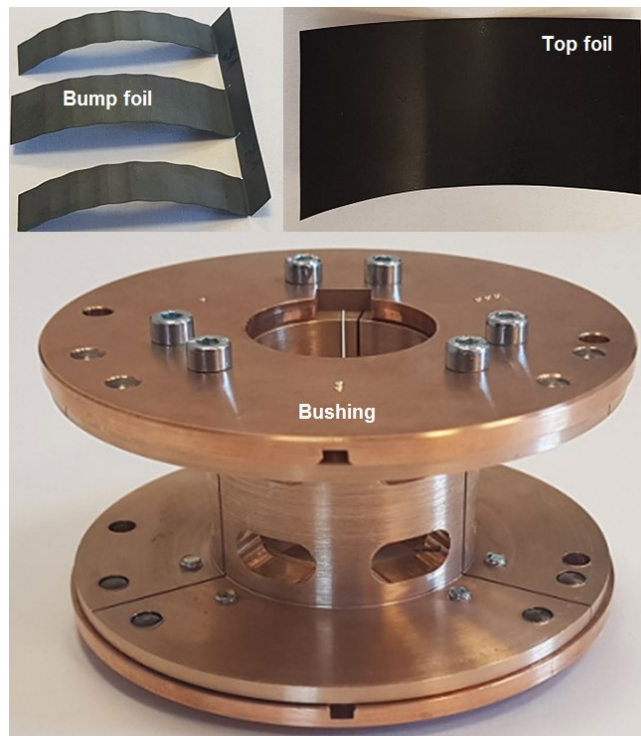
Figure 2: Main structural components of the GFB before their assembly.
