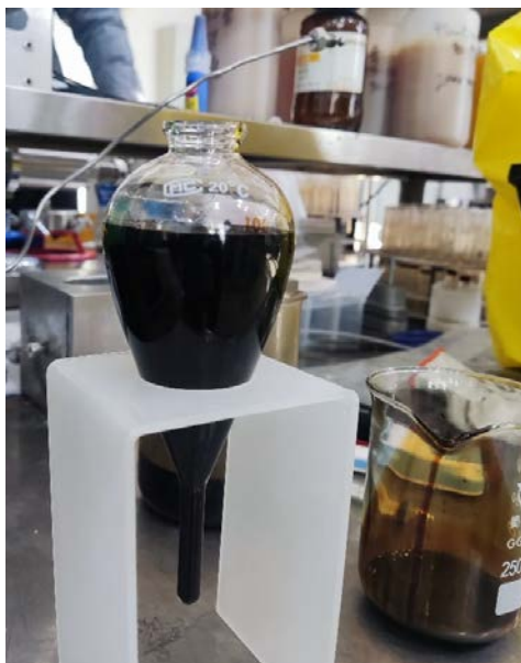
(a) The oil sample was filled into the conical flask.
