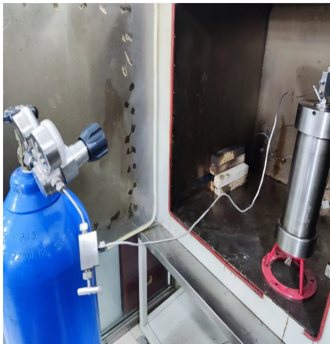
(c) Pressurizing the intermediate container using nitrogen gas.
