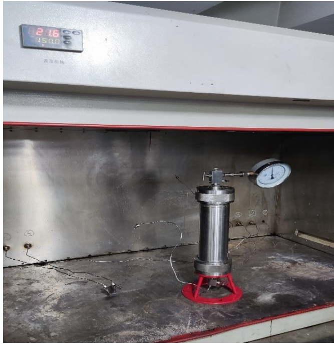
(d) Setting the environmental temperature using a thermostatic chamber.
