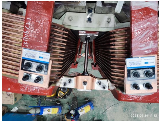
Fig. 2 Installation Diagram of Temperature Measurement Sensor
