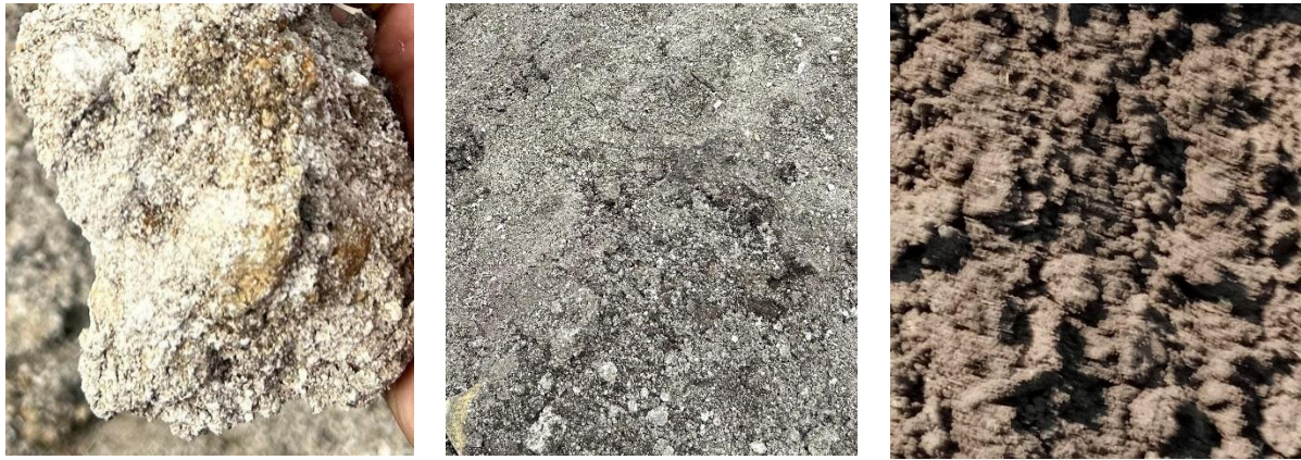
Figure 1: (a) Crusted sodic soil sample with salt efflorescence from Mehkar, (b) granular sodic soil surface at Butkheda, and (c) dispersive sodic clay structure under sunlight at Khorad Sawangi, Mantha
