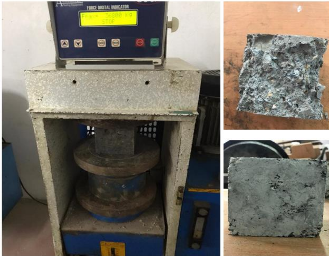
Figure 3. GPC specimen and testing mechanism
