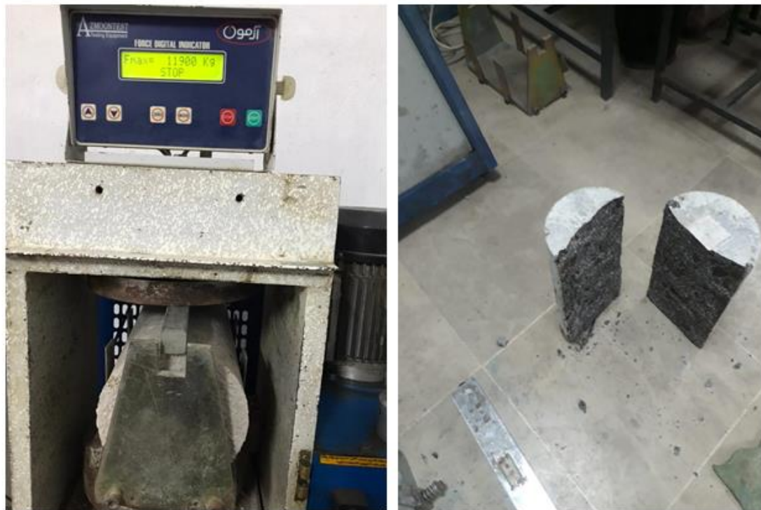
Figure 6. Tensile strength set up
