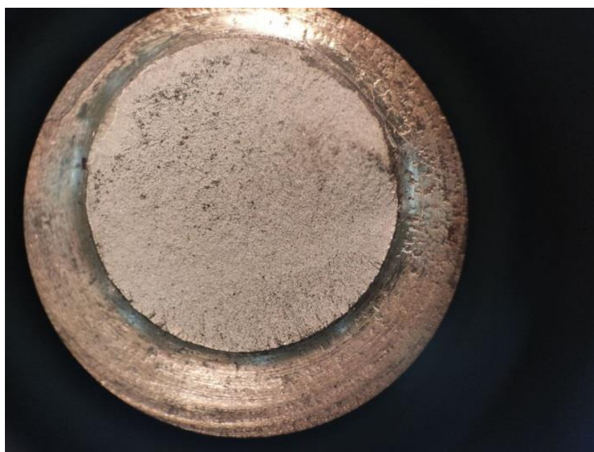
Fig. 12 Optical photomicrograph (x20 magnification) of the fracture surface of a rotary bending fatigue test specimen at a stress of 360 \text{ N/mm}^2 and Ra = 0.075 after 48623 cycles of C 45 steel quenched at 850^\circ\text{C} and tempered at 200^\circ\text{C} ( H_v=247 ).
