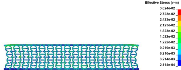
Fig.9.b. 11.7 J Impact Response of HEX_0.5CON
