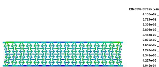
Fig.10.c. 26.49J Impact Response of HEX_0.7CON
