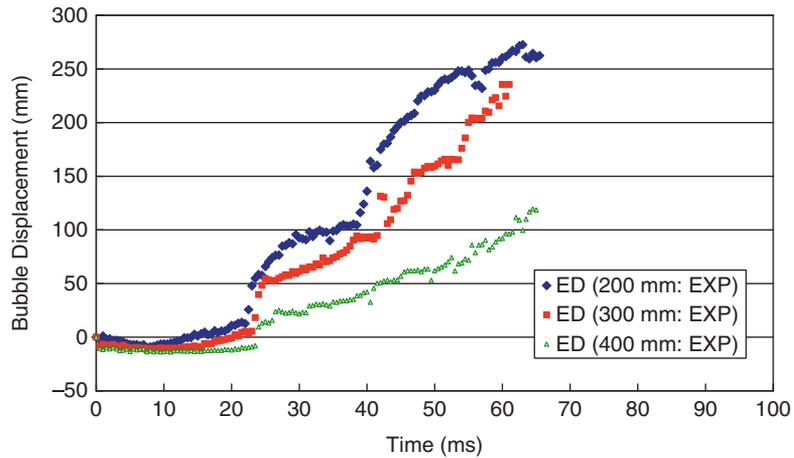
Figure 8 Displacement history about the center position of the bubble gas.
