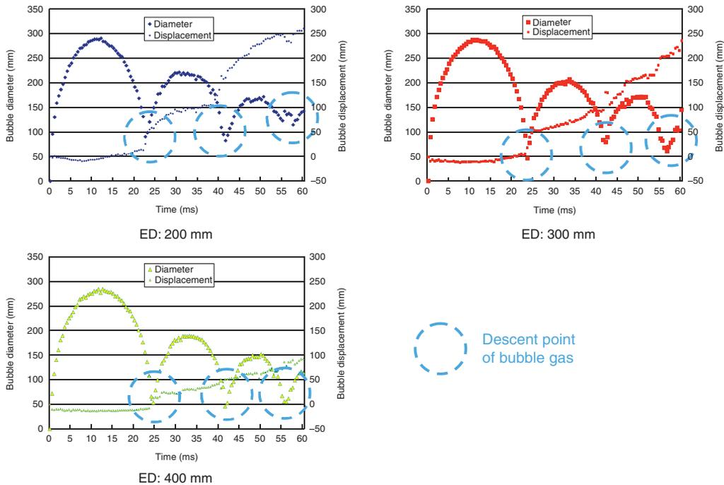
Figure 9 Diameter of the bubble gas and descent of bubble gas.
