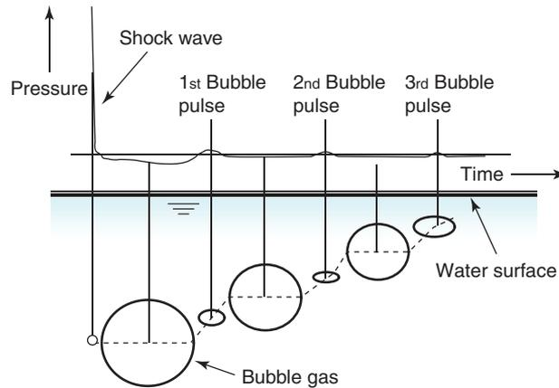
Figure 1 Schematic illustration of underwater explosion phenomenon.
