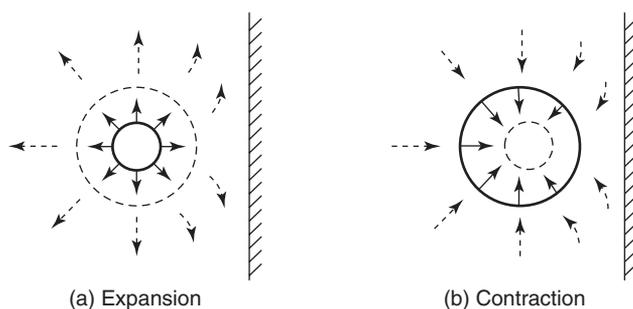
Figure 6 Behavior of the bubble gas near the rigid body wall.
