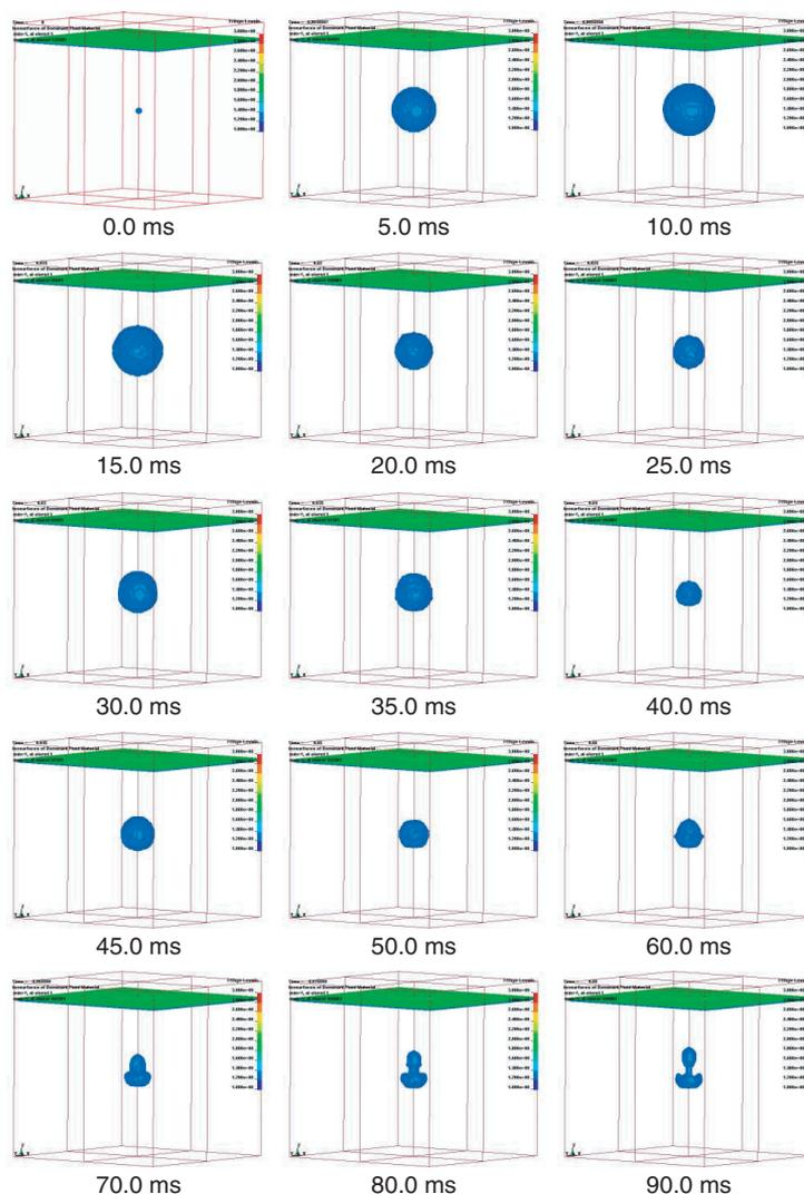
Figure 11 Image of bubble gas obtained by numerical simulation in case depth of explosive is 400 mm.
