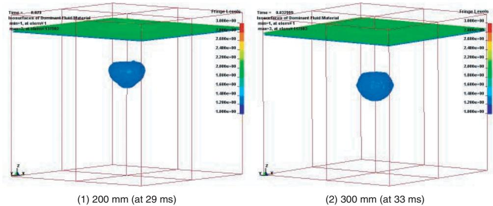
Figure 12 Image of bubble gas at 2nd cycle when depth of explosive is 200 mm and 300 mm.
