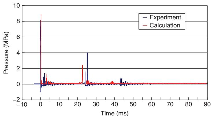
Figure 16 Comparison of the pressure measurement results.
