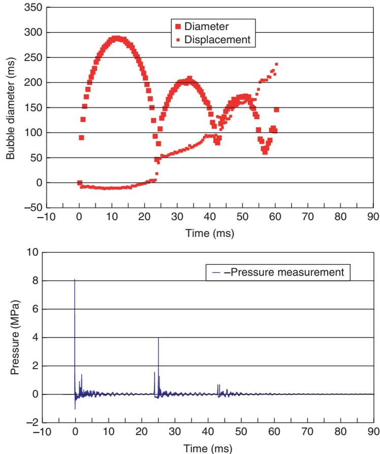
Figure 10 Comparison of pressure measurement result, maximum diameter of bubble, and displacement of bubble gas.
