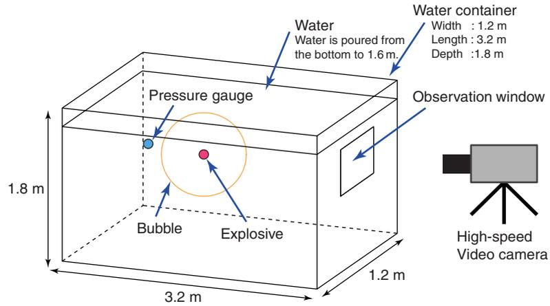
Figure 2 Experimental setup.
