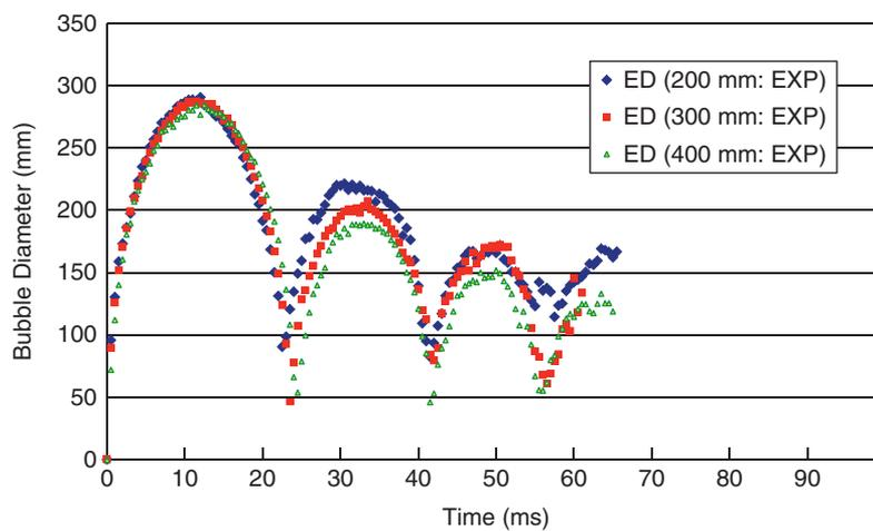
Figure 7 History of the diameter of the bubble gas obtained in the experiment.
