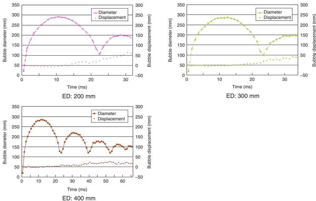
Figure 13 Diameter of bubble gas and descent of bubble gas obtained from numerical simulation in each condition.
