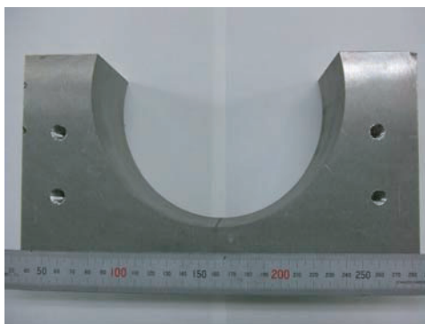
Figure 5 Experimental device for the optical observation of underwater shock wave converging
