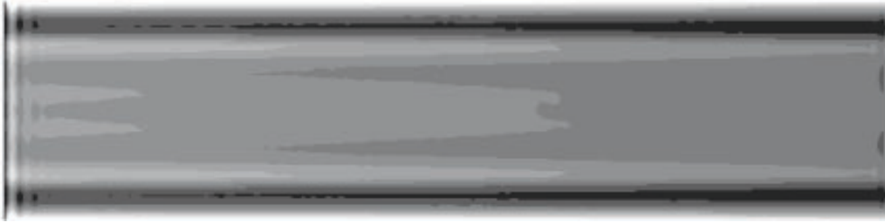
Figure 6. Typical density field along the nanochannel. L = 60\sigma , h = 6\sigma , \varepsilon_v = 0.79
