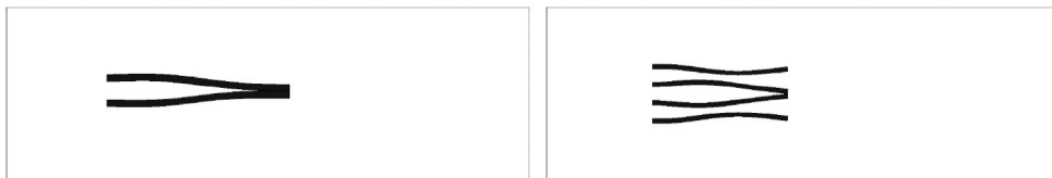
Figure 5. Touch of plates due to high inflow velocity.
