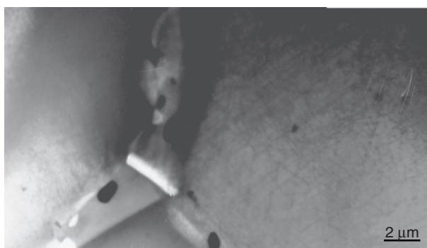
Figure 2 Microstructure of the supersaturated solid solution before compression. Zn particles are present at grain boundaries.
