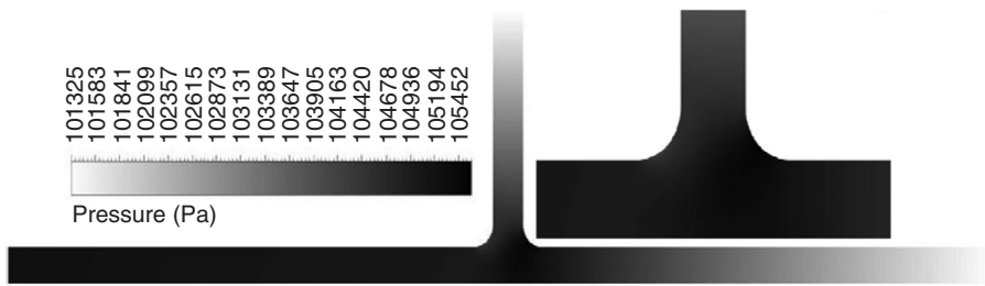
Figure 4 Field of pressure along the T joint.
