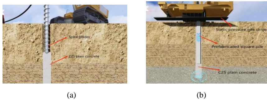
Figure 1: (a) Guiding-hole construction (b) Static pressure pile construction
